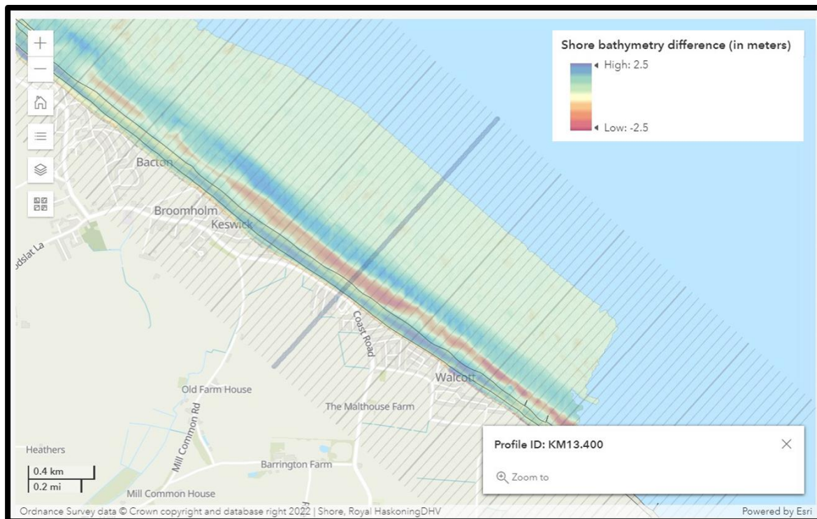
Example of difference analysis of sediment at Bacton, denotes reprofiling of sediment into the lower sub tidal near shore.
